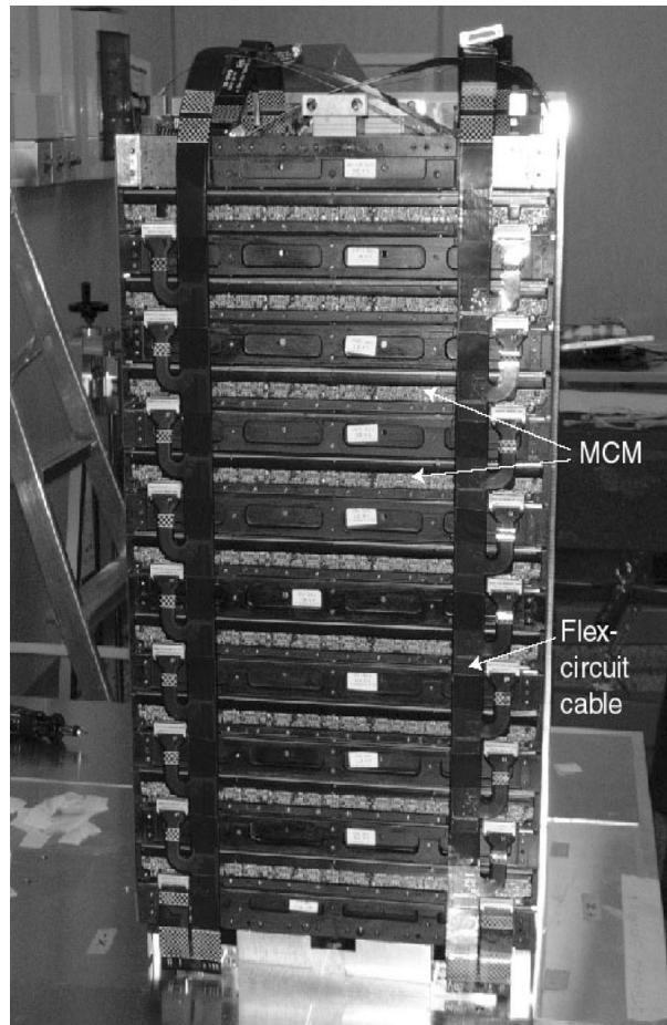
Figure 3.18: Inverted view of one tracker tower module without a sidewall
