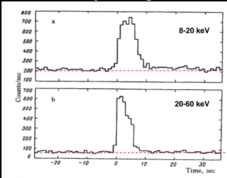
Observations of a cosmic gamma-ray burst on 23 July 1992 with the WATCH instrument on the *Granat* observatory
