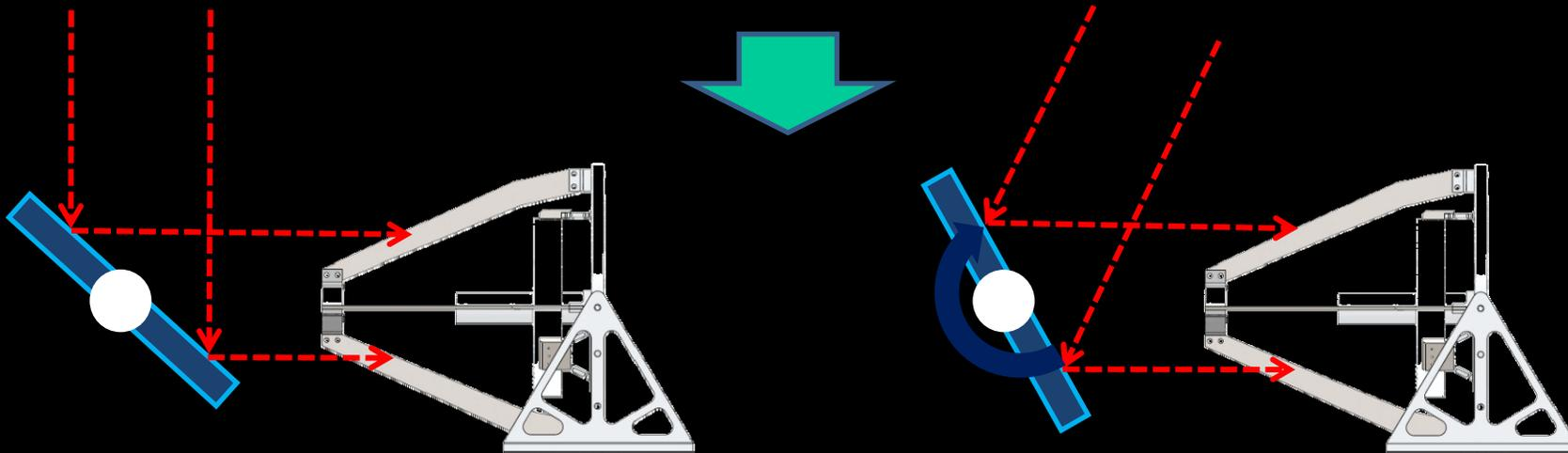
In UFFO-p, we move the optical path, not the spacecraft with fast slewing mirror system → much faster (NEW Concept)
