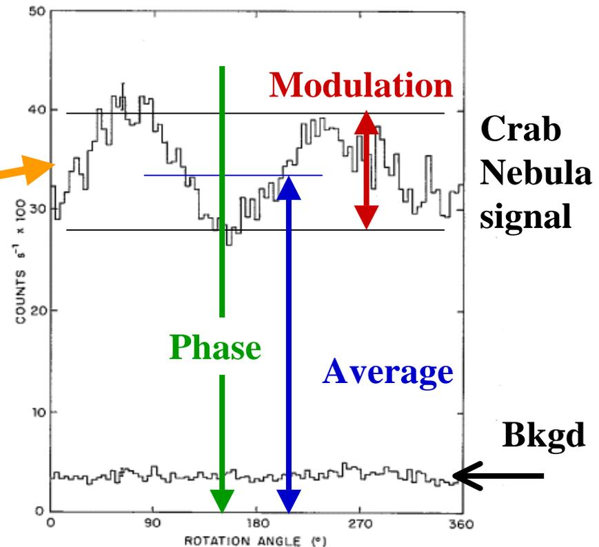
FIG. 2.—Average modulation curves obtained with both detectors at 2.6 keV during (upper curve) observations of the Crab Nebula and during (lower curve) observations of the Earth-occulted instrumental background.
