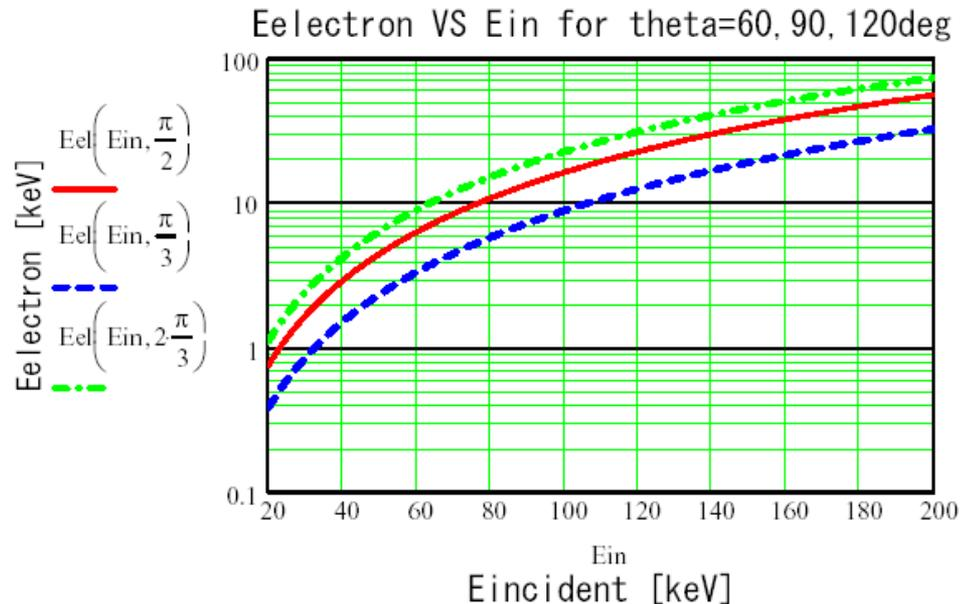
Energy of the recoil electron vs. the incident energy for the 3 theta's.
