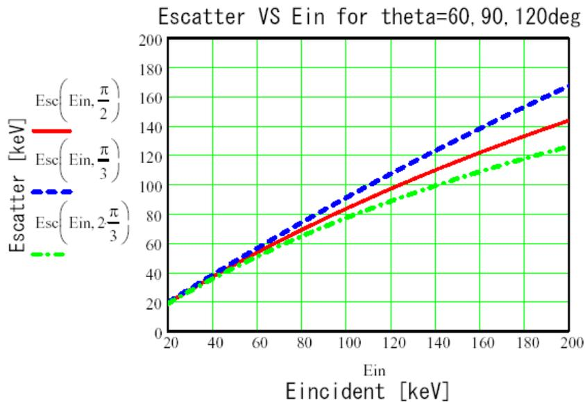
Energy of the scattered photon as a function of the incident energy for theta=60(blue dash), 90(red solid), 120deg(green dot-dash).
