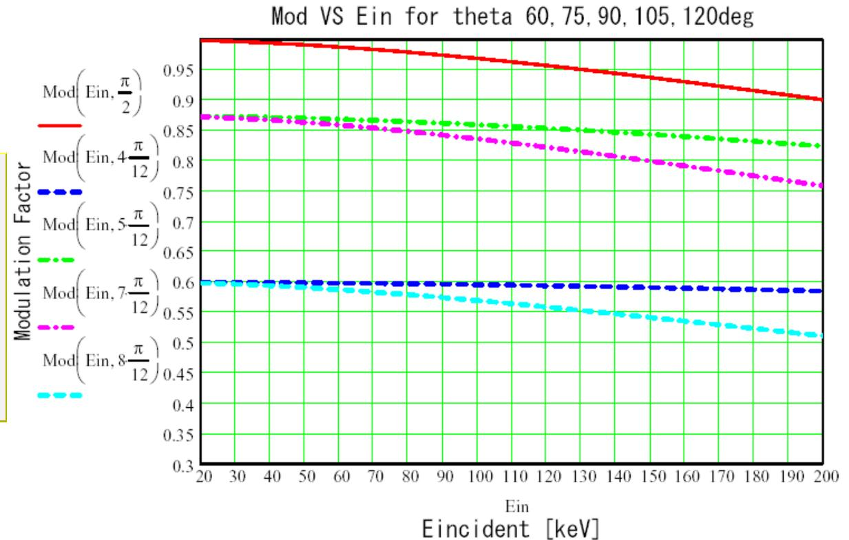
**Fig.5-3 Modulation factor of Compton scattering vs. the incident energy: scattering angle (theta)=60deg(blue dash), 75deg(green dot-dash), 90deg(red solid), 105deg(purple dot-dash), 120deg(magenta dash).**
