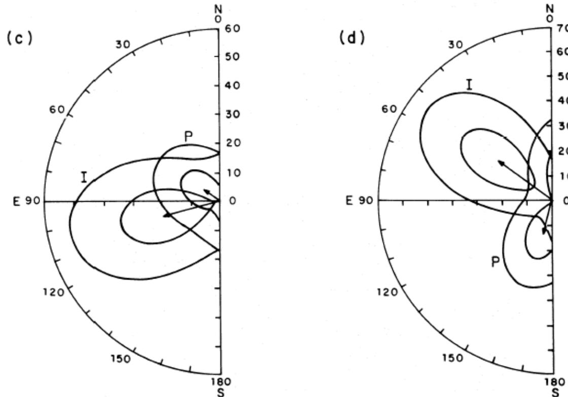
FIG. 2.—The polarization vectors at 2.6 keV for the four pulse phase ranges of the primary (P) and interpulse (I): (a) total pulse, (b) central pulse, (c) leading edge, and (d) trailing edge. Surrounding the vectors in order of increasing size are the 67% and 99% confidence contours. The radial scale is the polarization in percent.
