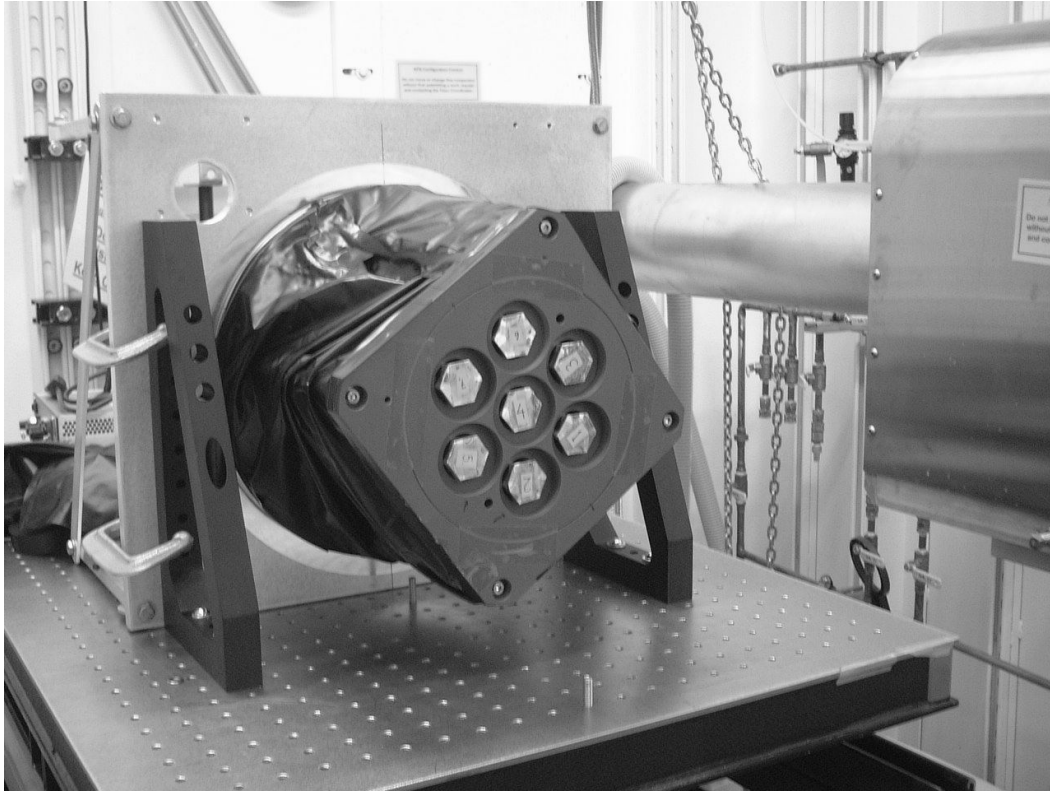
Fig. 3. A photograph of the PoGO prototype mounted on the rotation stage attached to the experiment table.
